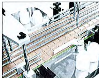
Reject station for 1st container rejection on every start up & parameter change
