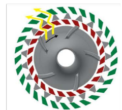
Variable shear intensity thanks to direction-changing homogenising mode [clockwise]
